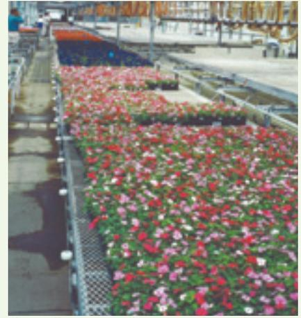
The pallet system from Rough Brothers is a network of bench supports with rollers, transport lines and conveyors. The bench tops, or pallets, glide on top of the system.
